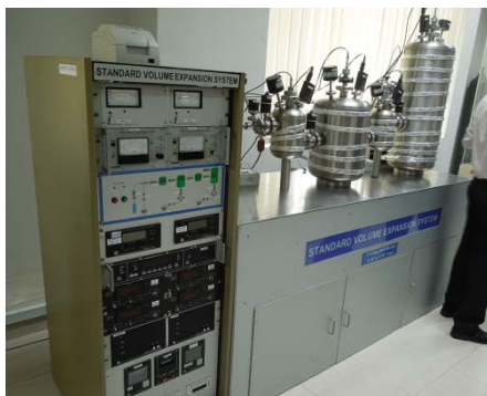
Fig. 3.: Volume expansion system for calibration purposes
