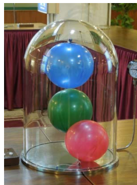
Fig. 4.: One experiment at the interactive exhibition: initially deflated balloons expand when the surrounding pressure is reduced
